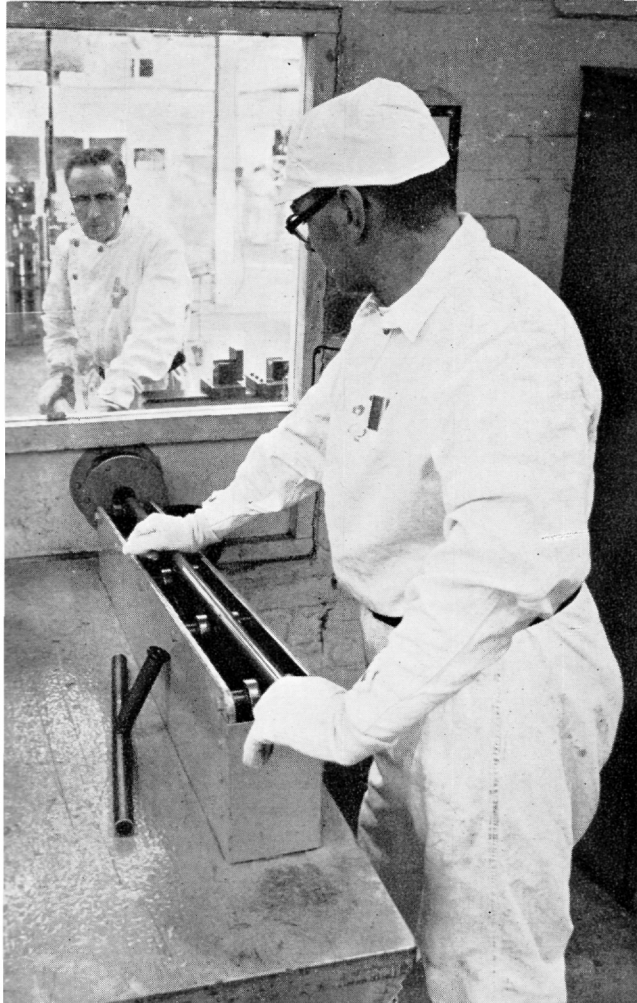
The fuel element production line at Springfields. To prevent uranium contamination of the outside of fuel elements, no uranium is handled or allowed uncovered in the canning section of the line.
