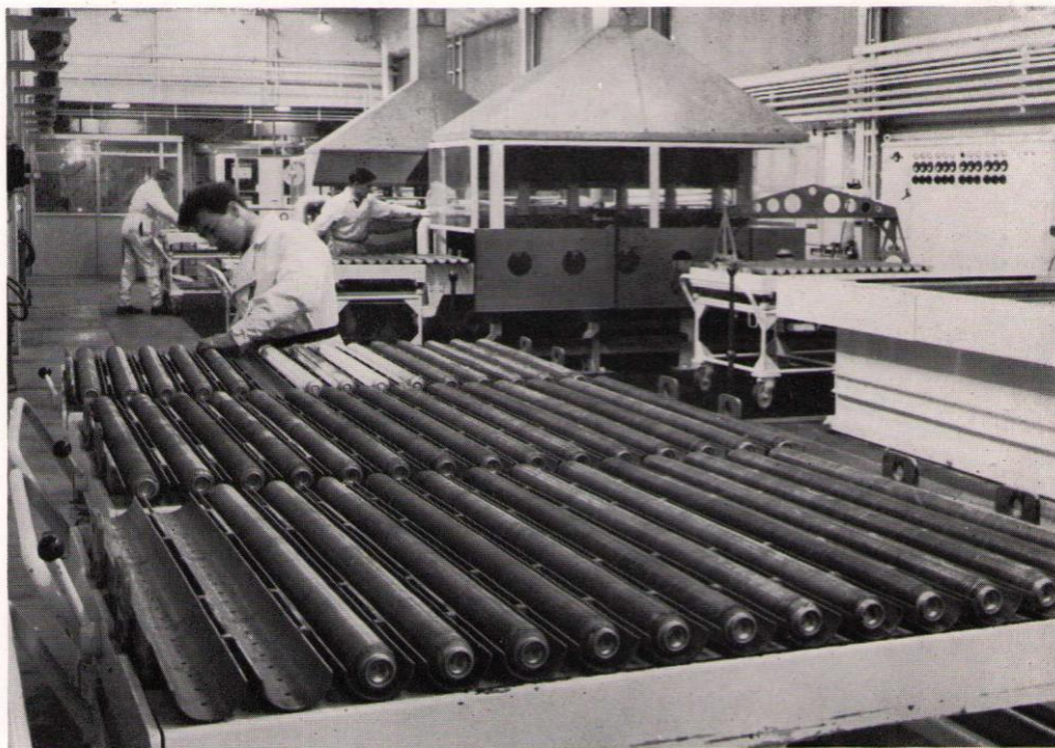
SPRINGFIELD, NEW FUEL ELEMENT CANNING LINE. The second Springfield uranium plant was opened on 7th June, 1958. It is designed to satisfy all the fuel element demands of the first civil power reactors, and to provide uranium and uranium oxide fuel elements for experimental and prototype reactors.
