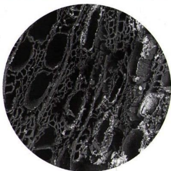
Wood from the Mary Rose analysed by new scanning electron microscope
