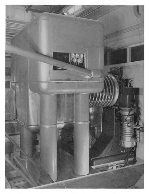
The polarized proton source installed on the Proton Linear Accelerator.
