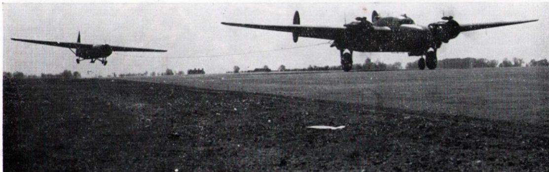
An Albemarle tug aircraft taking off with a Horsa glider, which becomes airborne before the towing aircraft.
