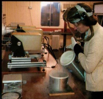
Liquid nitrogen calibration for the microwave radiometers at Chilbolton Observatory
