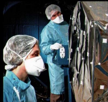
Thermal model of the JWST MIRI instrument MLI (inset) and photo-type MLI blankets during preparation for thermal balance testing
