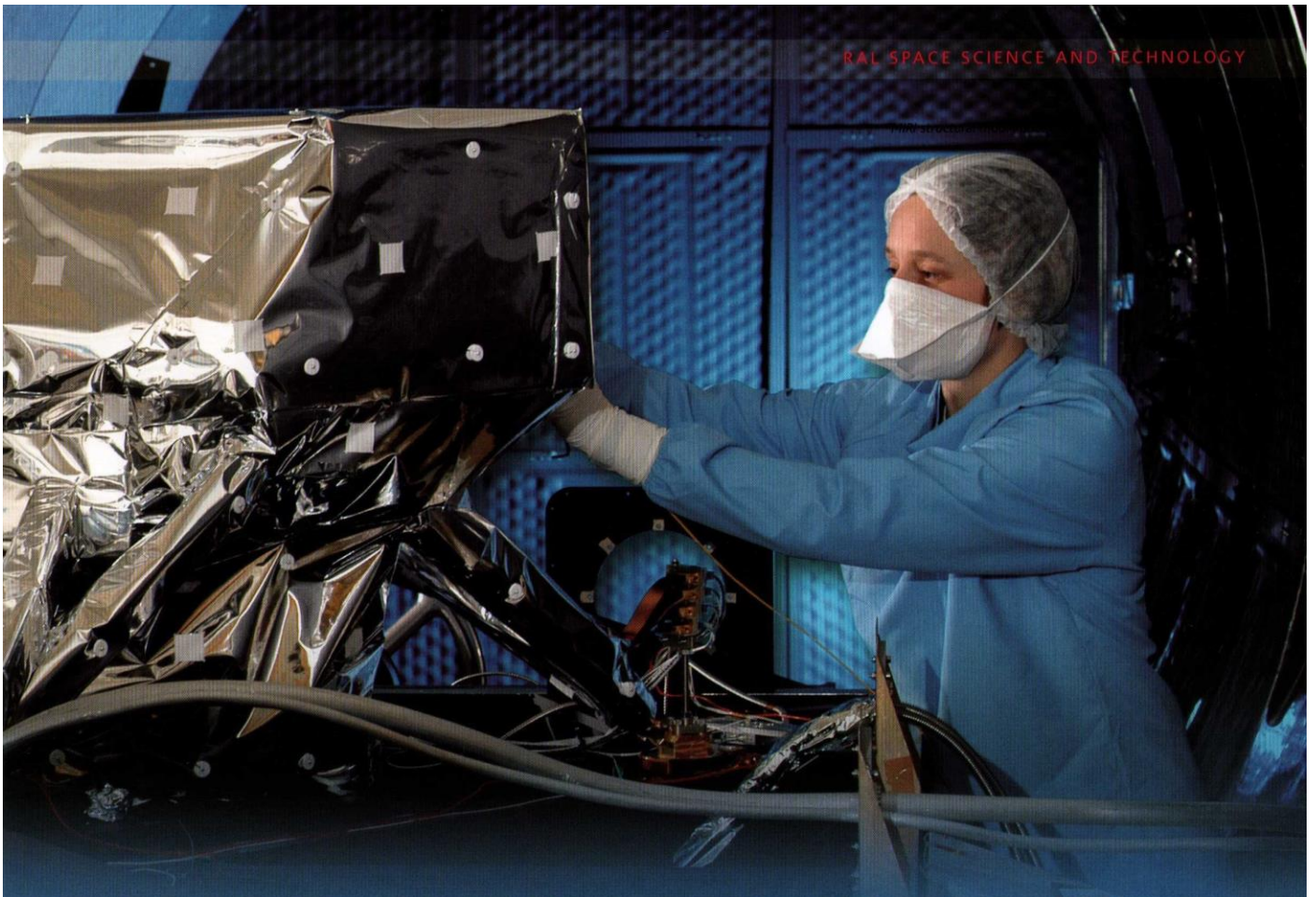
A member of the Thermal Engineering Group prepares a prototype of the Mid-Infrared Instrument (MIRI) of the James Webb Space Telescope (JWST) for cryogenic testing in SSTD's Space Test Chamber
