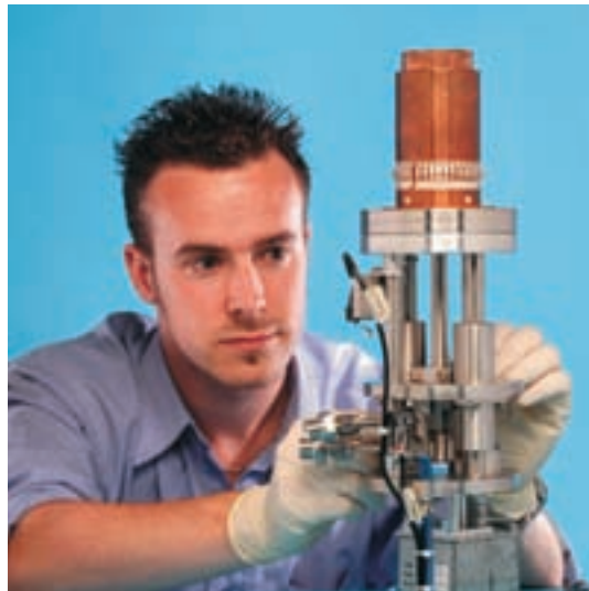
Chris Benson from the ISIS Project Engineering group working on the tuner for the ISIS radio-frequency quadrupole accelerator, 2004.
