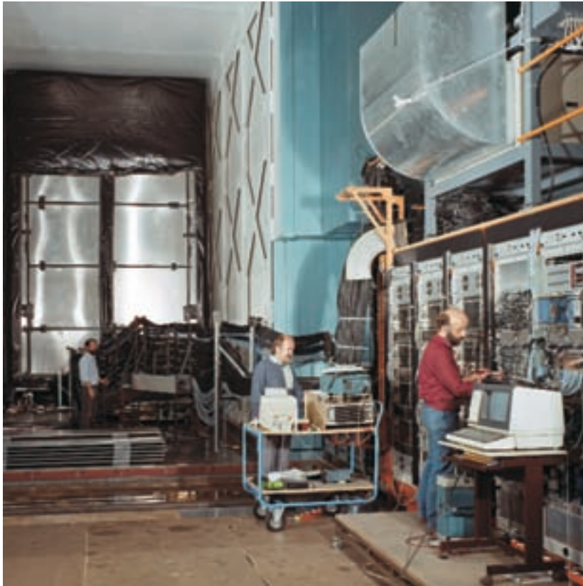
❖ KARMEN neutrino facility at ISIS, 1988. Karlsruhe-Rutherford Medium Energy Neutrino (KARMEN) was an experimental neutrino physics programme investigating charged current and neutral current neutrino nucleus interactions.
