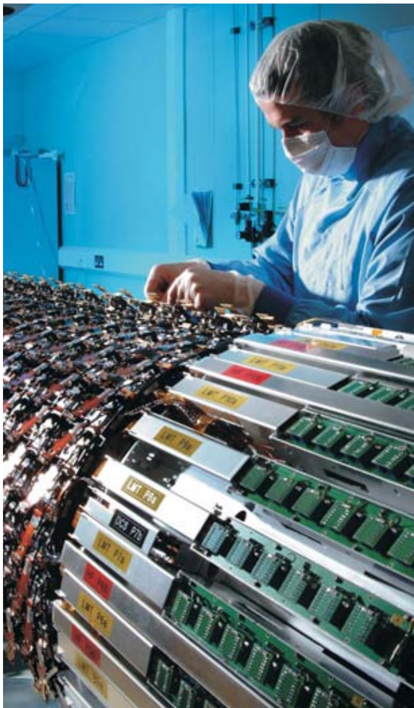
Impressive views of ATLAS cavern side A, 2007. The detector module built at RAL is one of the principal elements of the ATLAS inner detector.
