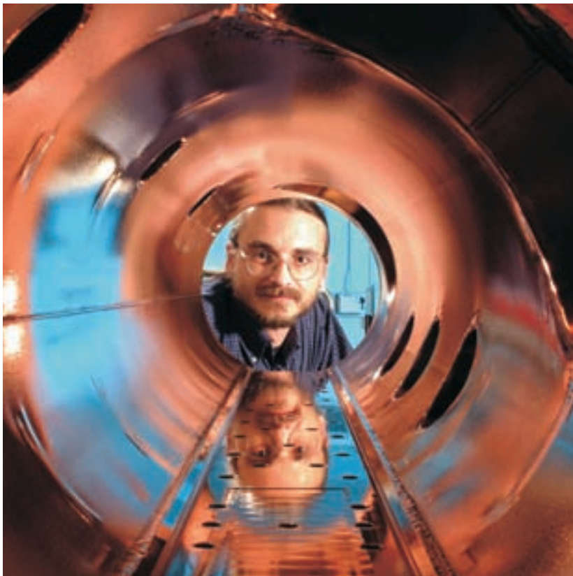
Alan Letchford looking down the inside of the vacuum vessel of the ISIS radio frequency quadrupole (RFQ) accelerator. This 4-rod RFQ was installed on ISIS as an upgrade for the existing but ageing Cockcroft-Walton pre-injector, 2003.
