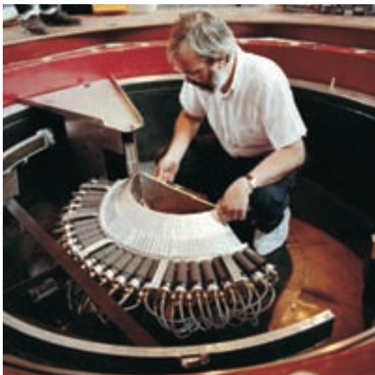
⚡ Dr Colin Carlile, Instrument Scientist on IRIS installing a new detector bank. From 2001 to 2006 Dr Carlile was Director of the Institut Laue-Langevin.
