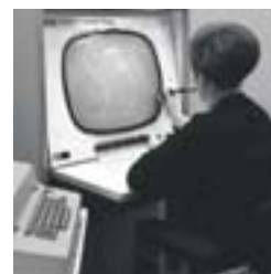
⋄ Computer controlled graphics display used to scan data from bubble chamber experiments in Atlas, 1970.
