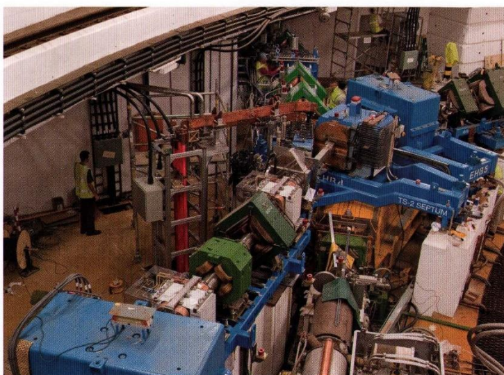
→ The new beam extraction area in the ISIS synchrotron will take proton beams to the ISIS Second Target Station Project. The extracted beam flies over the synchrotron and forks left to Target 2 and right to Target 1
