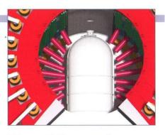
Eighteen radial beam ports allow neutrons to travel out to the instruments.
