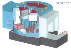
The 12m diameter, 7m high steel and concrete structure closely follows the existing target station design. The interior contains the target and moderator assembly surrounded by a stainless steel containment vessel filled with helium. For maintenance, the target assembly can be withdrawn into a service area with remote handling equipment.
