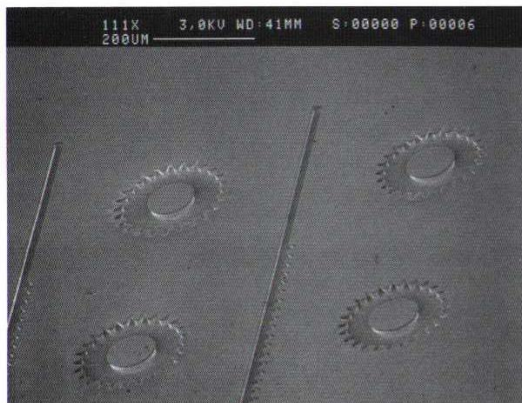
Fig 4.1.1 SEM photograph of some typical gold features on a beryllium membrane LIGA mask
