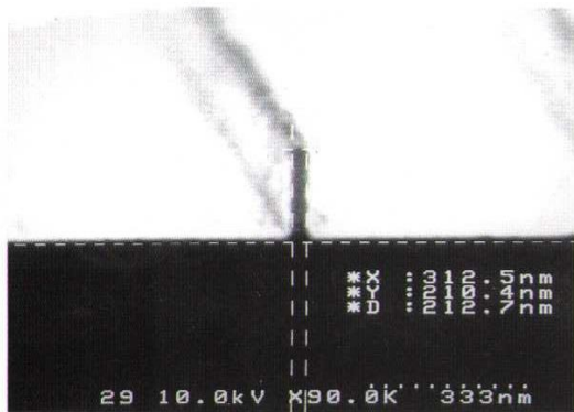
Fig 5.1.1 30 nm AZPN114 negative resist lines with 7:1 aspect ratio
