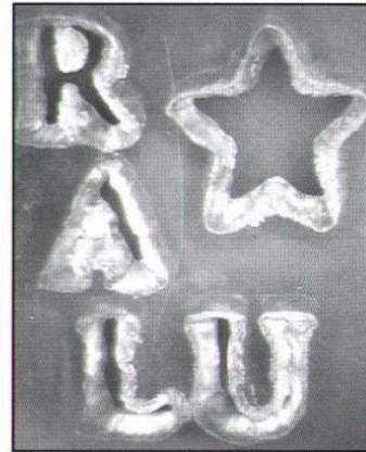
Fig 2.1.3 Photograph of a laser burn print in perspex from above kinoform, size 11 x 14 mm
