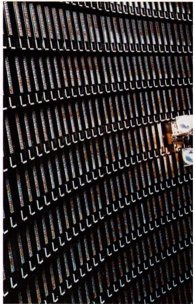
Vast amounts of information are stored at the Atlas Centre including data. Once data tapes are loaded they are selected by robots as requested by
