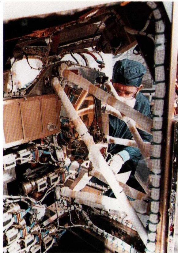
Space instruments are built and tested under very clean conditions as the slightest speck of dust could impair the performance of equipment which cannot be cleaned once launched.
