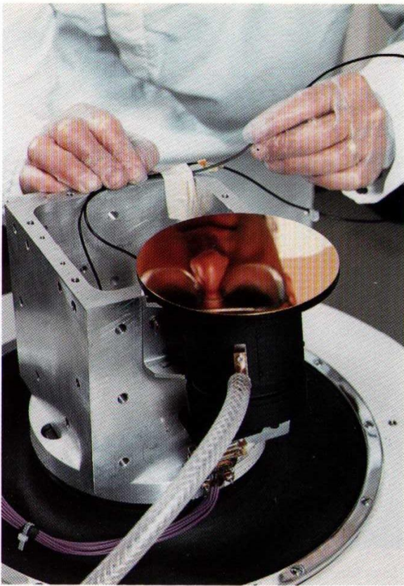
This highly polished mirror is part of the ATSR project to measure the temperature of the sea surface from 500 miles up in space. The mirror will rotate six times a second throughout the three year mission.
