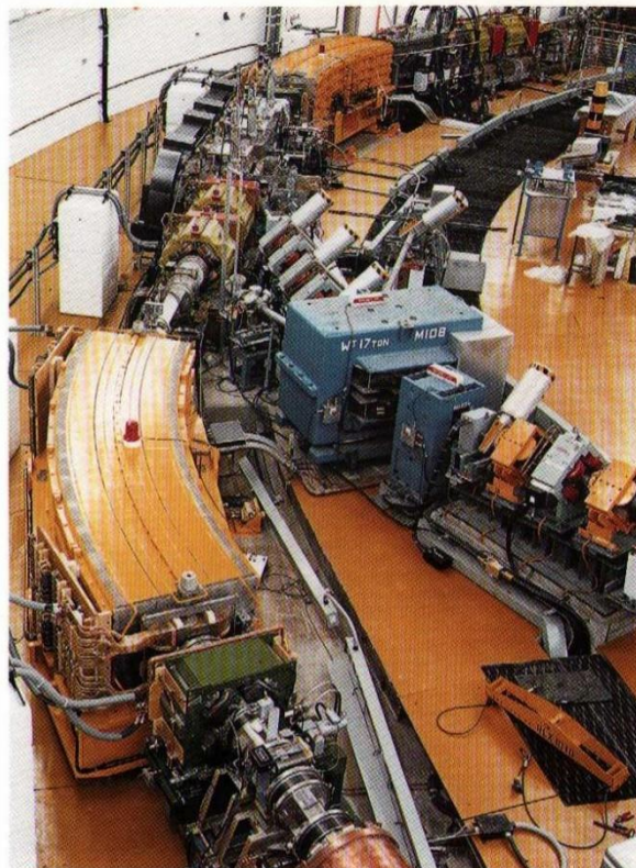
This 52 metre diameter circular machine (a synchrotron) is used to accelerate protons before they are diverted down a tunnel to collide with a uranium target.
