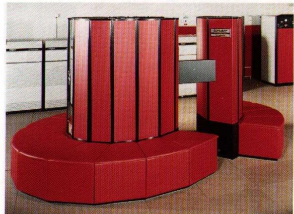
The Cray supercomputer is built in this unusual shape to minimise the length of electrical connections, thereby increasing its speed of operation.
