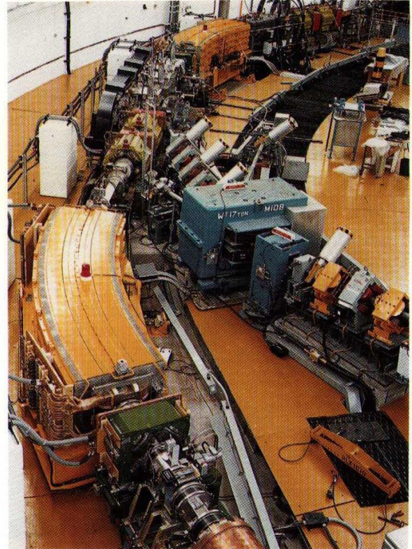
This 52 metre diameter circular machine (a synchrotron) is used to accelerate the particles before they are diverted down a tunnel to collide with a uranium target.
