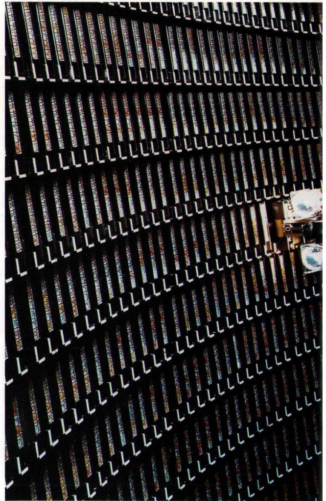
Vast amounts of information are stored at the Atlas Centre including data robots select tapes at the request of computer users.
