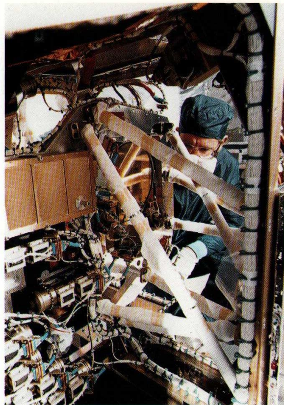
Instruments for space are built and tested under very clean conditions as the slightest speck of dust could impair the performance of equipment which cannot be cleaned once launched.
