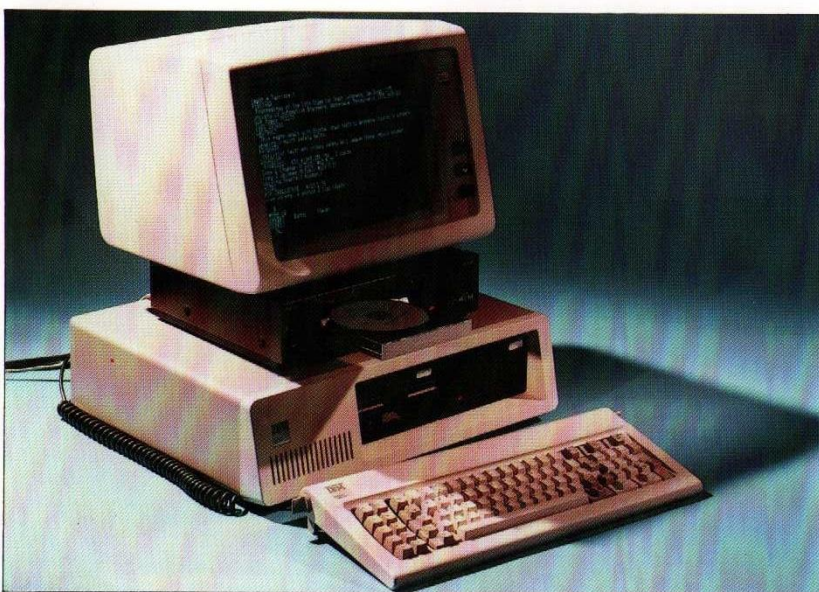
A prototype system for compact disc based information retrieval using STATUS.
