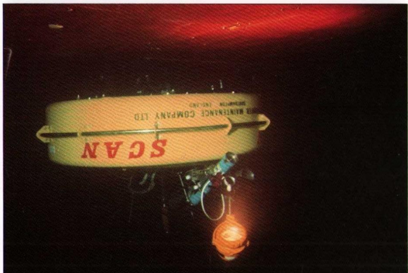
SCAN-A remotely controlled submersible developed at Harwell.
