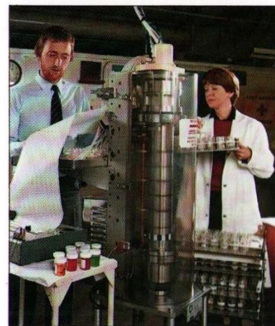
Harwell's electrophoretic separator, now licensed to CJB Developments Ltd. Its main application is the separation of macromolecules such as the anti-haemophilia Factor VIII from blood plasma.
