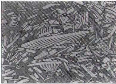
Section of solidified intermediate level solid waste – Magnox swarf in concrete.
