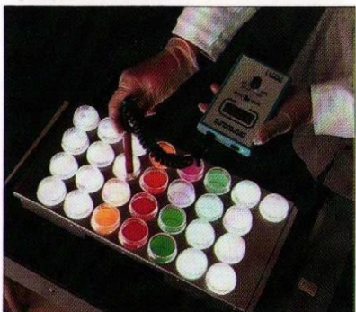
Making measurements on dyes fractionated by the BIOSTREAM continuous electrophoretic separator.
