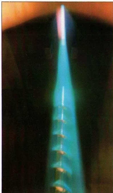
A large feed screw from a plastic injection moulding machine being implanted with nitrogen ions.
