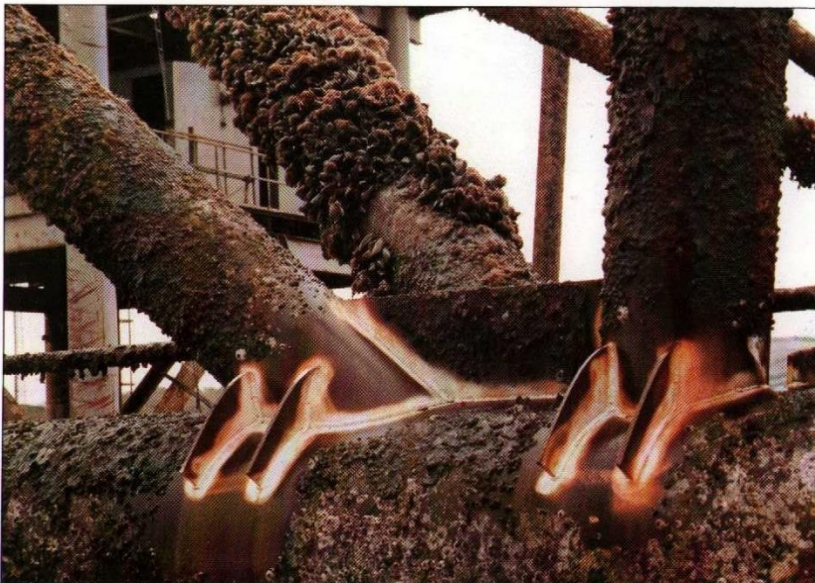
Marine fouling: part of a gas platform removed from southern North Sea, with joints cleaned for weld inspection. Normally this is done underwater.
