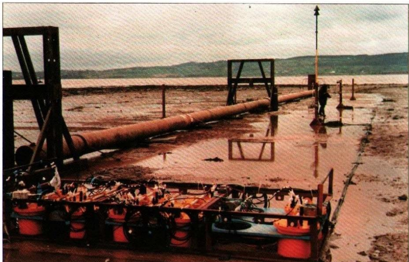
A test rig for measuring vibrations of pipeline spans induced by currents near the sea bed. The rig, at Shepperton in the Severn Estuary, is shown at low tide when it was accessible for setting-up, adjustment and maintenance. The instrumented fifty metre length of 500mm diameter pipeline was submerged beneath a maximum of six metres of fast flowing water at the high tide condition.
