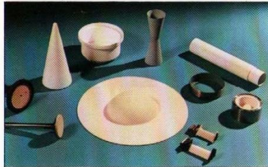
A range of engineering components either ceramic coated or fabricated directly by plasma spraying processes.
