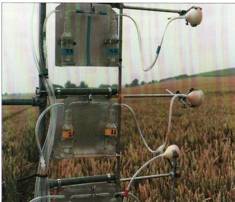
Measuring the vertical profile of ammonia vapour over a wheat field to determine the rates of emission and deposition.
