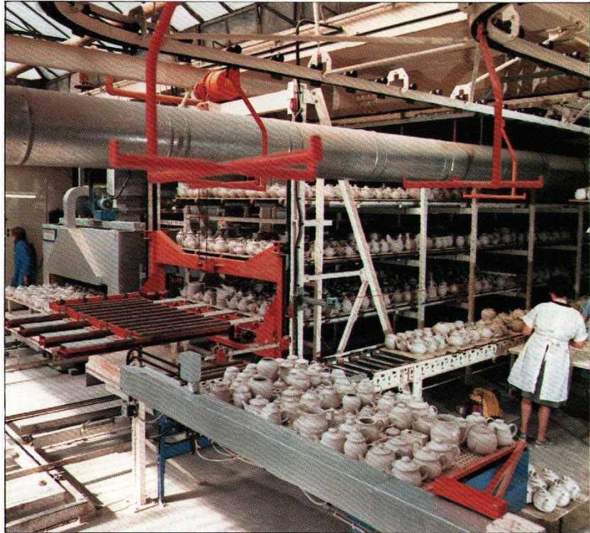
The adoption of a fast firing system introduced at James Sadler & Sons Ltd, Burslem (the UK's largest manufacturer of teapots) under the Energy Efficiency Demonstration Scheme has shown up to 65% energy saving.
