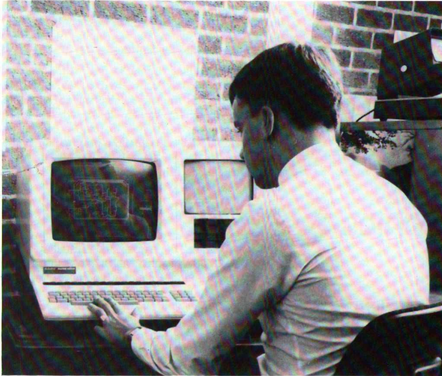
Fig 2.4 Wayne-Kerr Artworker used for testing printed circuit boards. (85RC5366)
