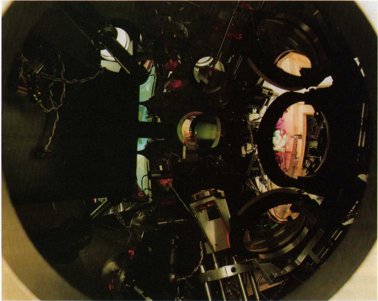
PLATE XIII The new VULCAN laser target chamber, showing optics to produce line-focus illuminations for x-ray laser research. (85 RC 5376)
