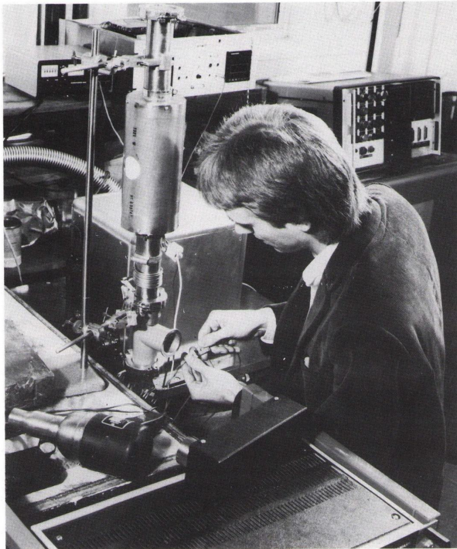
Assembling a gas 'flow-through' furnace for preparing ISIS neutron scattering samples
