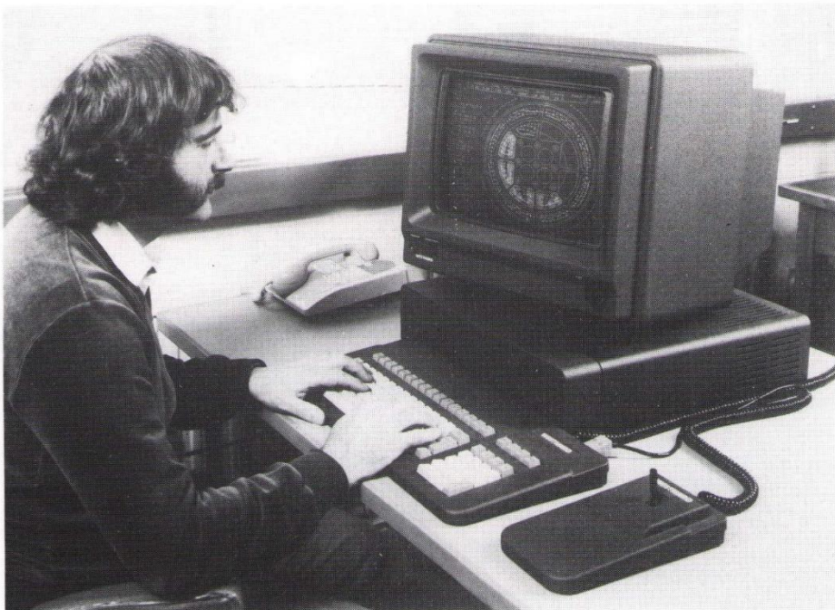
A craftsman adds machining instructions to a computer aided design before commands are transferred for computer controlled machining
