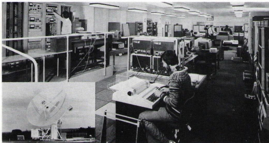
The Infra-Red Astronomical Satellite (IRAS) Control Centre at RAL Chilton. The antenna (inset) received scientific and engineering data transmitted from the satellite and sent control messages during the mission.
