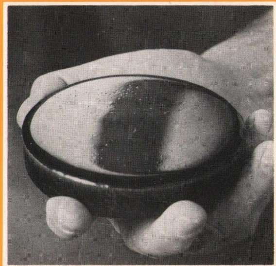
If all the electricity, domestic and industrial, used by one person in a life-time, were generated by nuclear power, the resultant long-lived radioactive wastes could be incorporated in a piece of glass this size.
