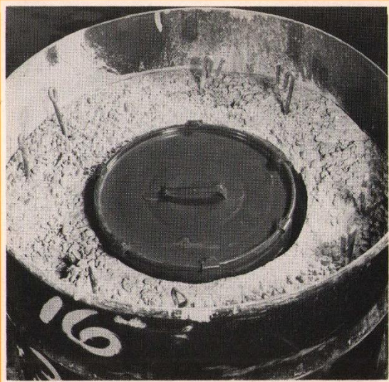
Drums packed with low active waste and fitted with concrete caps (not shown) are disposed of in the deep ocean. They must be strong enough to reach the sea bed intact. The inner drum is encapsulated in concrete – 90 per cent of the gross weight is packaging.
