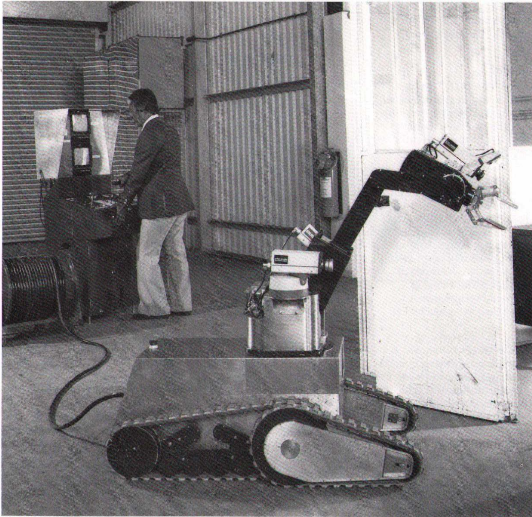
Figure 10 SPIDER: a remotely operated manipulator Developed for British Nuclear Fuels Limited
