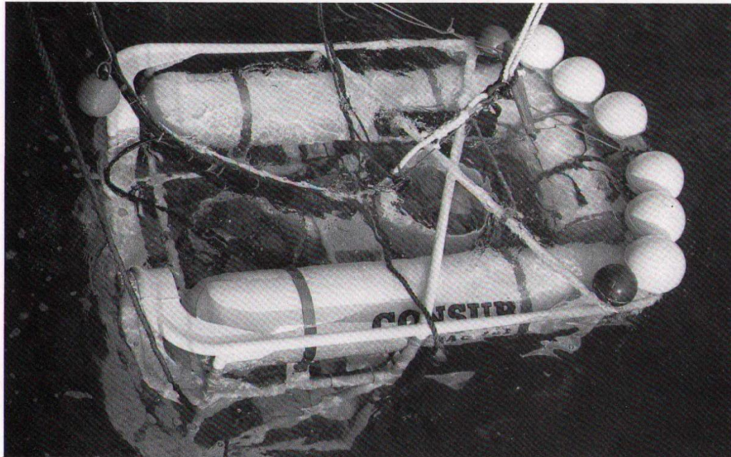
Figure 30 Unmanned submersible, 'CONSUB 1' An underwater rock-coring tool, built for the Institute of Geological Sciences by B.A.C. Ltd. (now part of British Aerospace), under MaTSU supervision. This submersible served as a prototype for the development of underwater engineering versions. Its design and construction were partly funded by the Ship and Marine Technology Requirements Board.
