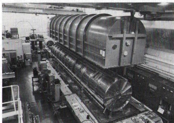
Fig 2. The RF cavity of the Nimrod injector with the vacuum cover raised.
