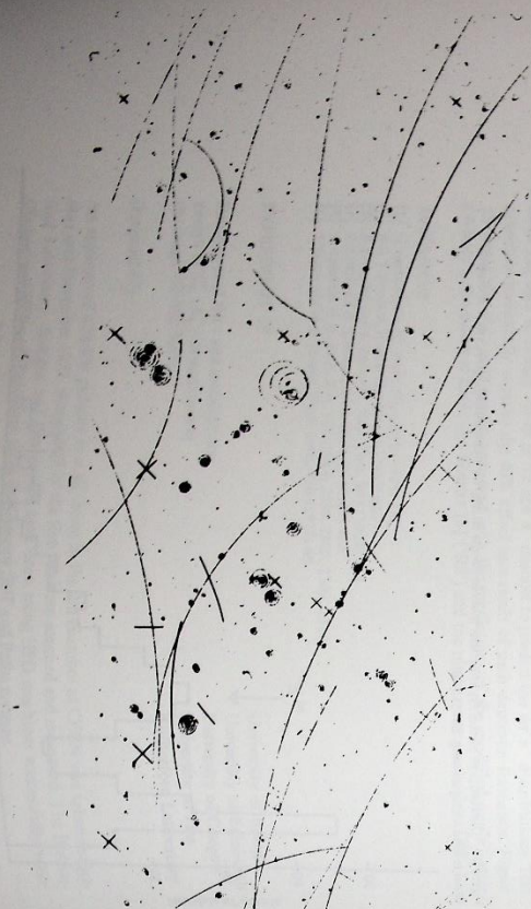
Figure 38. A frame from the K_S^0 exposure showing a semileptonic K_S^0 decay, a K_S^0 P \rightarrow K_S^0 P event with backward K_S^0 , and a K_S^0 P \rightarrow \Sigma^0 \pi^+ event with backward \pi^+ (and unseen \gamma ). The other recoil protons in the frame are due mainly to the neutron background in the beam, and the Compton electrons are due to soft photons leaking through the lead filter. Experiment 29 (15397)
