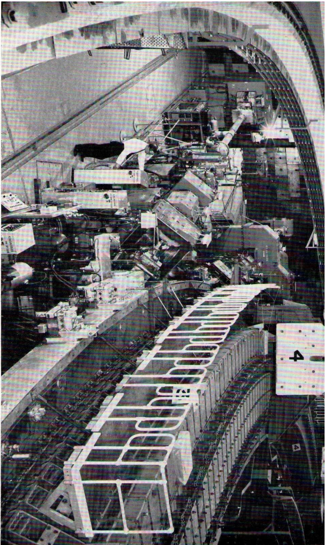
Part of the main ring magnet of Nimrod, in the region where the beam lines lead off to Experimental Hall 1.
