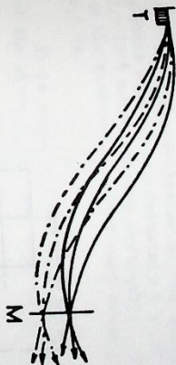
T - Target. M - Position of Magnet The chain linked lines represent the paths of protons which have lost energy in the target compared with other protons following the solid lines
