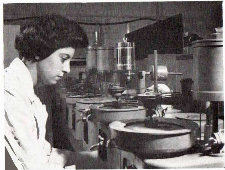
A Springfields laboratory assistant polishing specimens of can materials for microscopic examination
