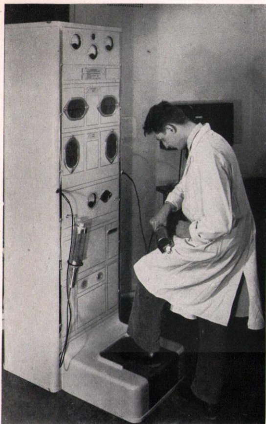
Using a personal health monitor. Clothing is being tested for contamination by a counter. The rubber-covered apertures are for hand testing. Footwear is tested by the stand.
