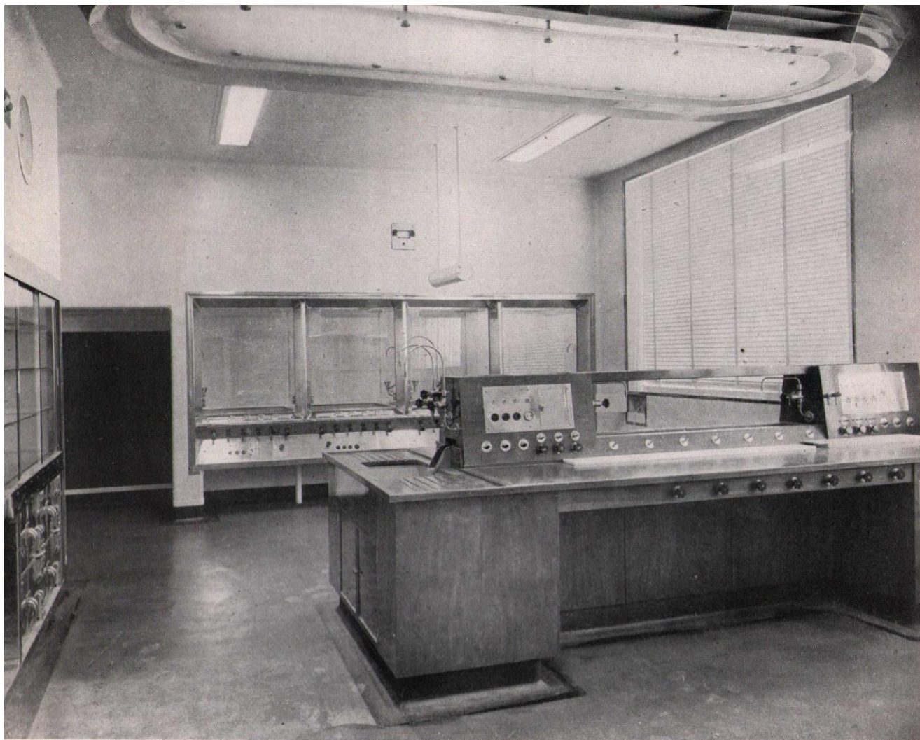
General view of a typical radiochemical laboratory. In the background is a fume cupboard for work with radioactive materials: left, glass-fronted store cupboards above lead lined storage space: right foreground, a bench for general work, in the ceiling above which is seen the ventilating air-inlet. Suspended from the ceiling, centre, is a cylindrical ionization chamber and, on the wall above the fume cupboard, an indicator for the measurement of radiation.
